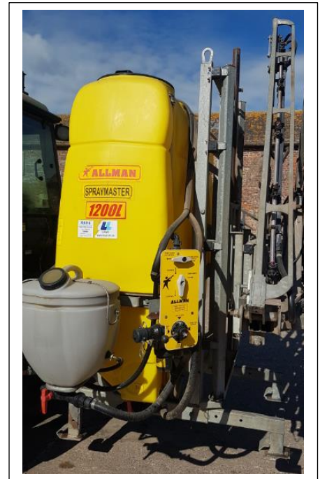
Allman 1200 litres spray – Electric controls, hydraulic boom folding
